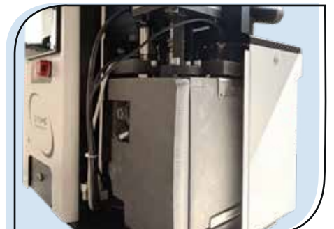
Minimal Maintenance. The front cover design provides easy access to all components, reducing maintenance time. While eliminating the tank significantly minimizes carbonization and nozzle blockages
